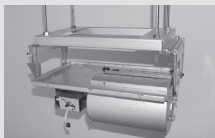
The hoisting tool has been removed and there is now enough space to connect the power and signal cables.
