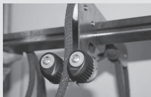
The self-locking pulleys on the hoisting tool make it possible for installation to be performed by just one person.
