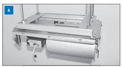
Finally the fog cannon is pushed to the metal plate and the screws can be tightened firmly.
