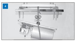
When the metal plate is firmly fixed, the fog cannon can be mounted in the two mounting brackets. We recommend our hoist tool to lift the unit from the ground (accessory).
