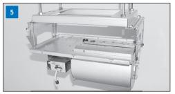
The hoist tool has been removed and there is enough space for connecting the power and signal cables.
