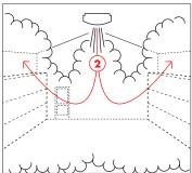
Total protection with fog is only about one thing: To deploy as much fog as possible into the room to ensure everything is covered as fast as possible. The number of fog cannon and their capacity is calculated in accordance with the architecture, and to the size of the room and furnishings.
