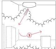
The direction and deployment of the fog in point protection is illustrated with the arrows. After the first, instant protection of the most valuable items (1) the fog spreads to the rest of the room (2). Walls and floors effectively make the fog "bounce" in all directions.
