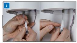
Fit the supplied new coupling in the hose. It is important that the hose is pushed all the way down over the coupling as shown.
